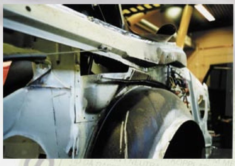
It is interesting to note the patchwork of metal sheets a prototype car is hiding underneath the surface...
