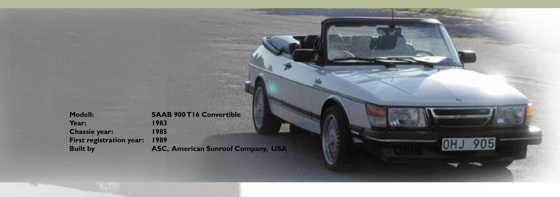
This car was built as the first 1983 prototype by ASC and the Swedish group under the supervisory of the head of the prototype department, Gunnar Arwidsson. The prototypes manufactured were done with a starting point from regular two doors 900i. They were solely built by hand (welded by hand using beams formed in a prototype metal adjustment machine). Thereafter a trial series was manufactured.
