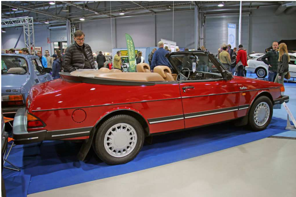
The roof neatly disappears behind the rear seats when it is opened.
